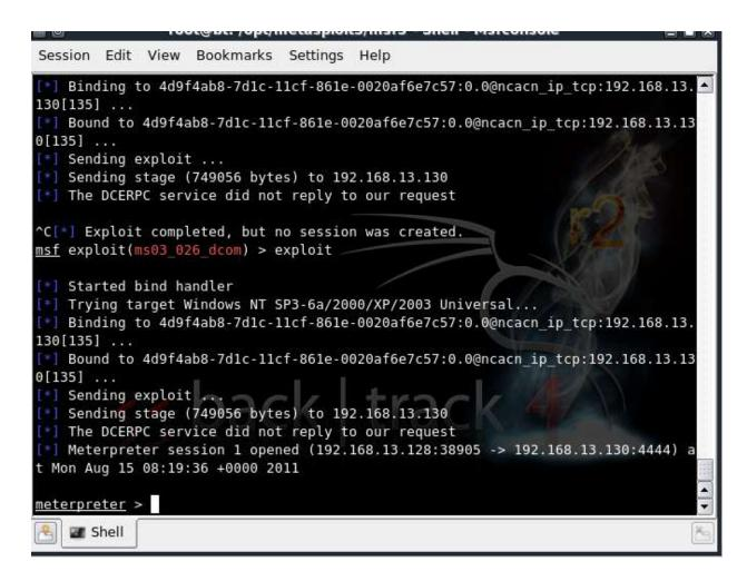
**Figure 4:** A Windows XP machine exploited by starting a meterpreter session
