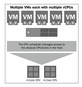
When all eight cores are available and the first VM makes a request, the CPU scheduler can provide the vCPUs with access to two pCPU cores, so the VM's operating system can operate as expected. The CPU scheduler can support simultaneous requests for only three more VMs running on this host. When the fifth VM makes a request, the CPU scheduler does not have access to any pCPU cores. Because the VM is unaware that it is virtual, it assumes it has access to the number of processors assigned.
