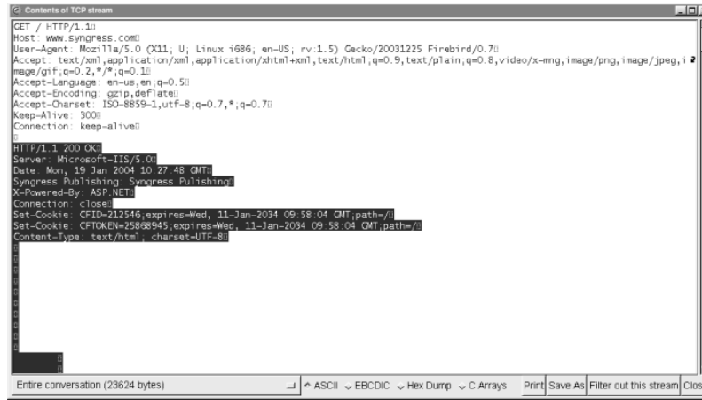
Figure 4.49 Contents of TCP Stream Window
