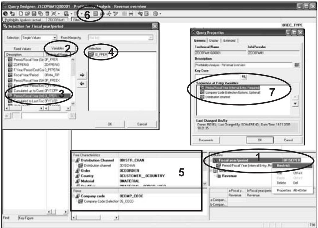
Figure 4.7 Inserting Variables in the Query Definition
