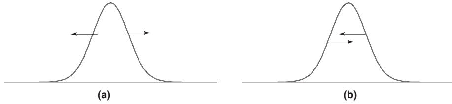
Fig. 5.24 SPM followed by negative and positive dispersion: (a) D < 0 , additional pulse broadening; (b) D > 0 , pulse compression.
