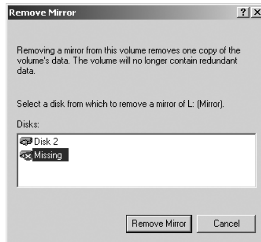
Figure 7-6. Removing the mirror from a failed RAID 1 volume
