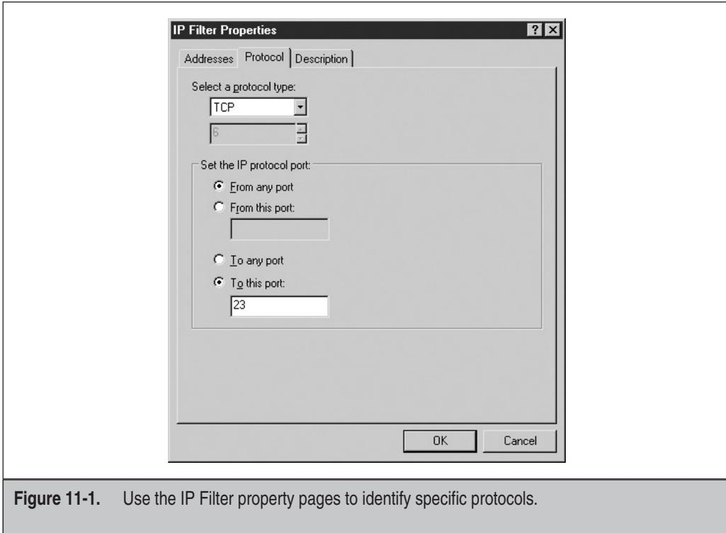
**Figure 11-1.** Use the IP Filter property pages to identify specific protocols.
