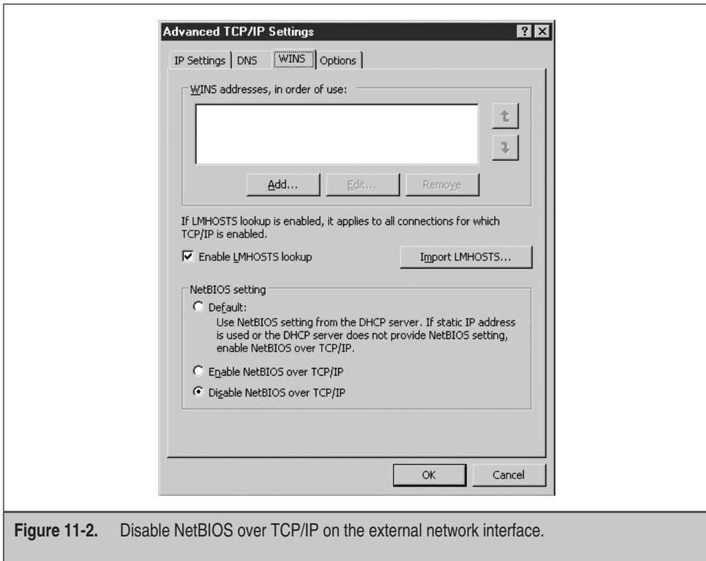
Figure 11-2. Disable NetBIOS over TCP/IP on the external network interface.
