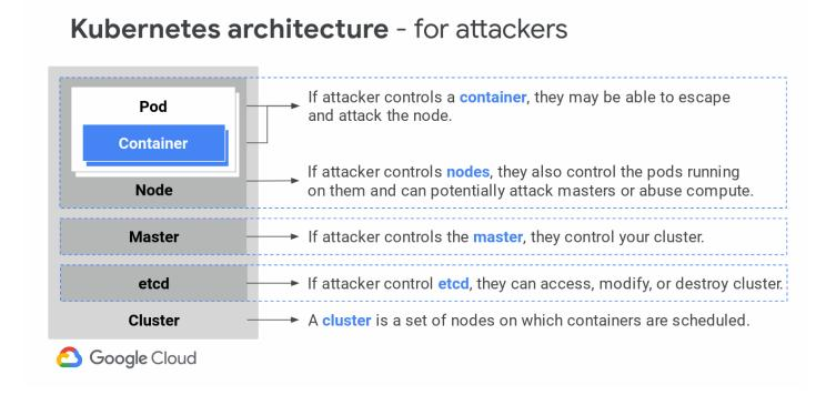
Multilayer Kubernetes security is a must because attackers can gain control throughout the Kubernetes stack, from a container to a cluster.
