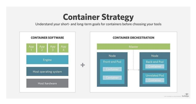
Left: The basic structure of container software, showing application components, the container engine for executing images, and host resources. Right: A Kubernetes cluster includes pods, which can encapsulate one or more containers; nodes, which host one or multiple pods; and the master, which creates and schedules pods.
