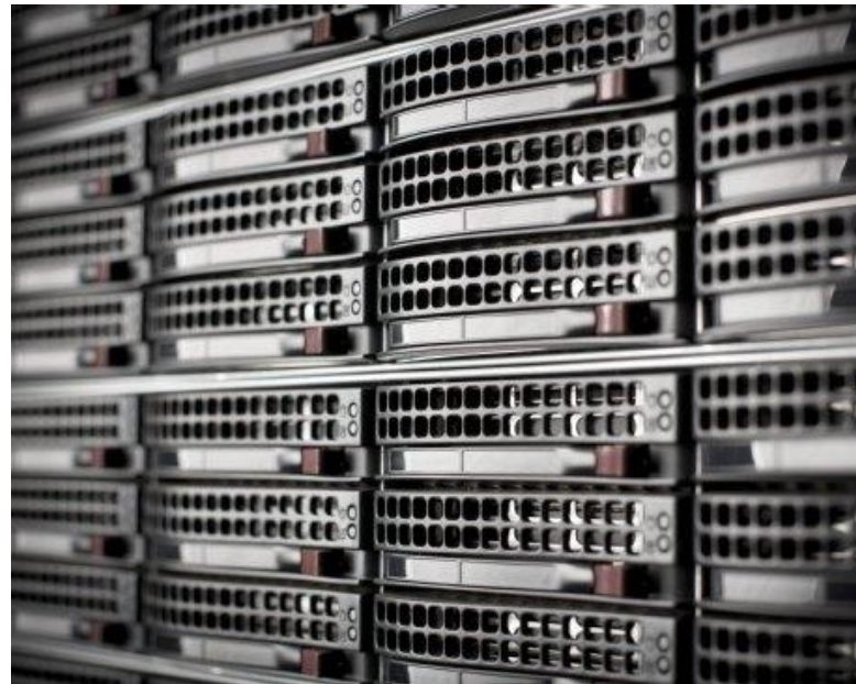
A blade server segregates processors, memory, I/O, disk, power and other components into separate modules.
