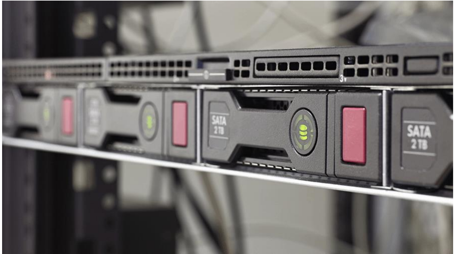
A rack server is designed to fit into a standard-size metal frame.
