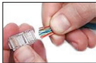
FIGURE 2-25 The clipped wires, ready for insertion into the RJ-45 plug.
