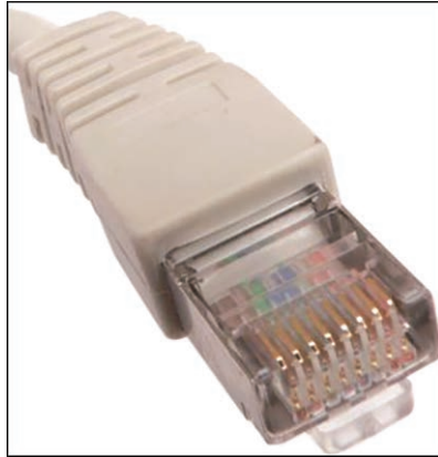
FIGURE 2-26 Wires pushed into the RJ-45 plug.
