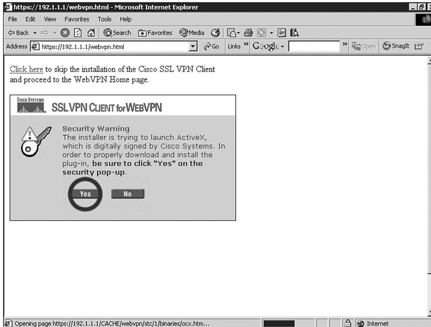
**TIP** For users in a group that use dialup for accessing the Internet, I would highly recommend that you choose the *Keep Cisco SSL VPN Client* option, because the downloaded software (SVC) is about 300 KB in size.
