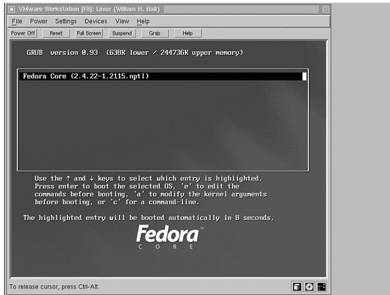
FIGURE 3.20 Boot Fedora with GRUB by pressing the Enter key or waiting 10 seconds.
