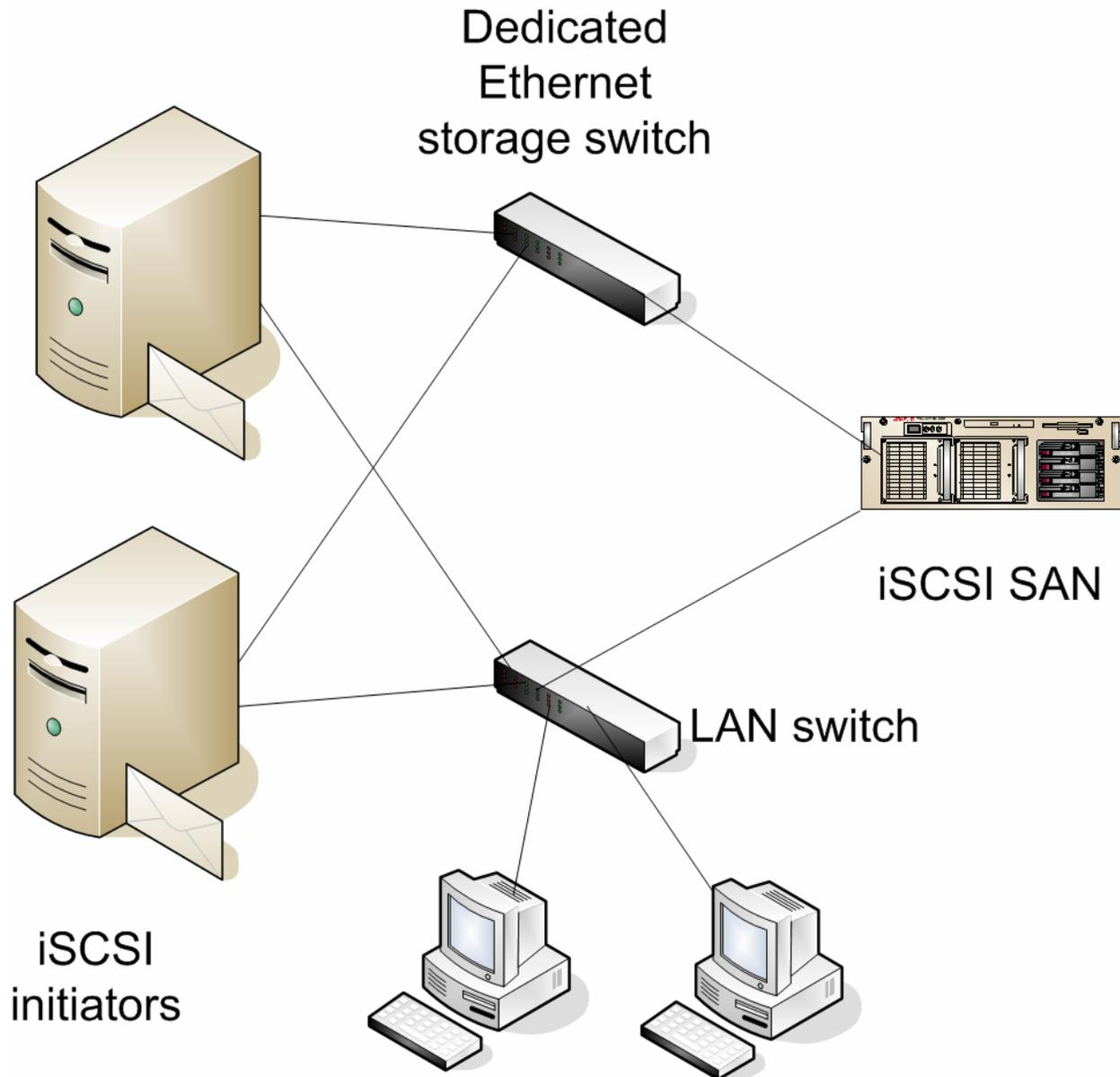
**Figure 3.3: Providing a dedicated network for iSCSI storage.**
