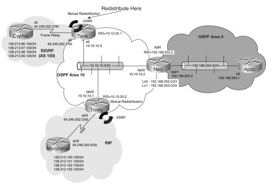
In this network, Router Tank is connected to OSPF area 10 and EIGRP AS 100. The entire OSPF network needs to know about the following networks:
