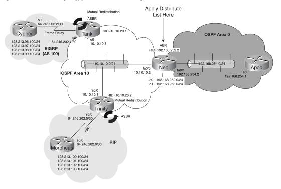
Figure 6-13 Network Topology for Distribute List Example
