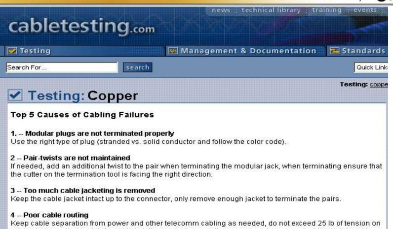
Keep cable separation from power and other telecomm cabling as needed, do not exceed 25 lb of tension on cables being pulled, watch for cable twisting and rubs on nails, screws, and even poorly drilled joists and studs.
