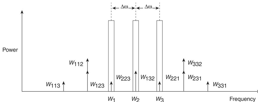
**Figure 4-13** Three Unequal Spaced Channels Generating Nine FWM Signals; None of the Generated Signals Falls on Top of the Original Signals
