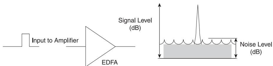
The noise is random in nature, and it is accumulated at each amplification stage. Refer to Figure 4-2.
