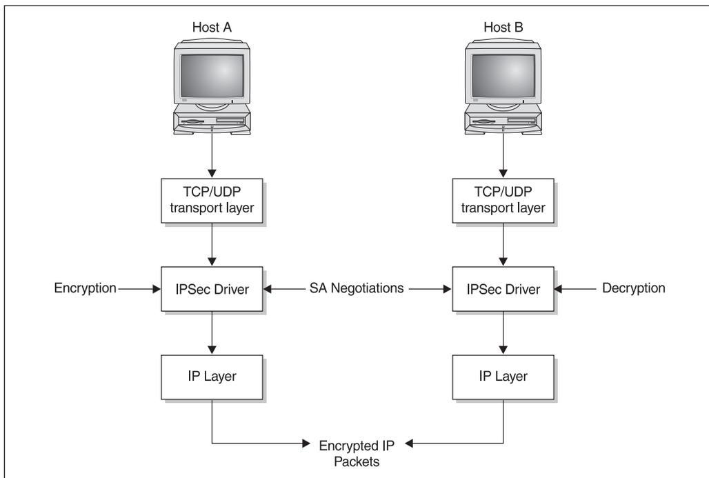
**Figure 9-11.** IPSec is set up between each communicating host pair.
