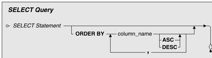
**Figure 4-10** The syntax diagram for the `SELECT` query
