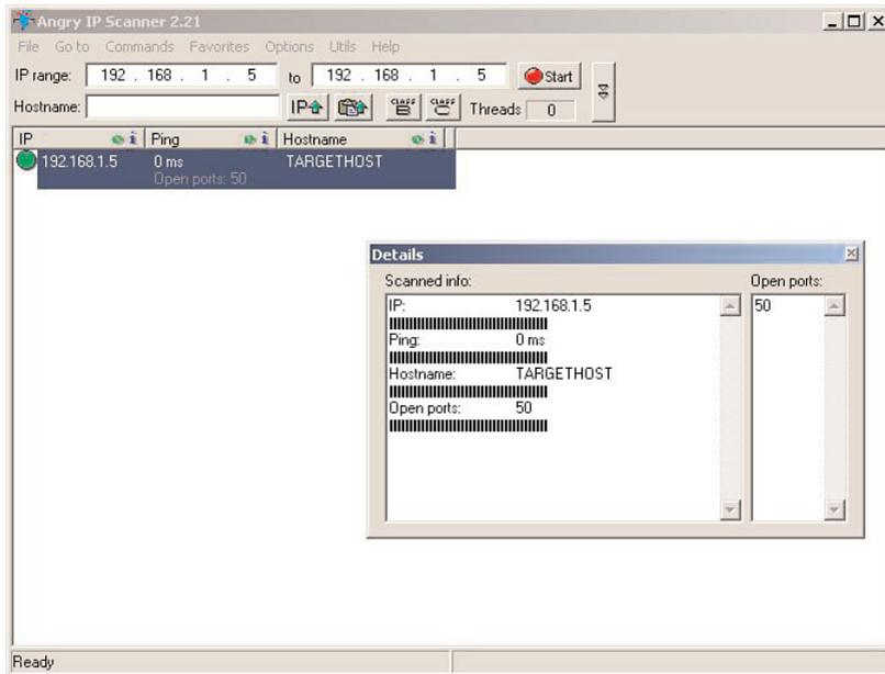
**Figure 2.20** Angry IP Scanner port scanner output
