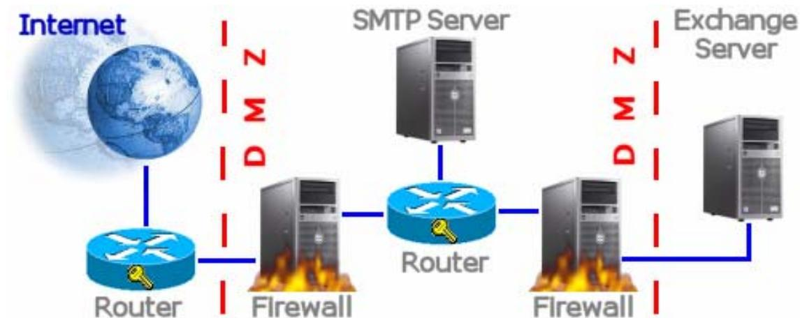
**Figure 1:** With this configuration, your Exchange Server's SMTP service never has to interact with an Internet SMTP server.
