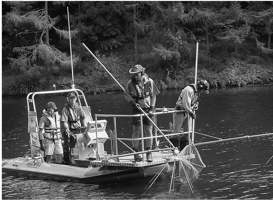
FIGURE 1.1 New Zealand's first electrofishing boat looks like something from a science fiction movie. But Waikato University's Te Waka Hiko Hi Ika is the first successful electrofishing boat. It has spectacular electronic prongs in front that dangle under the water and generate a 5 kilowatt pulsating electronic fishing field. Fish are temporarily stunned by the field and float to the surface. Pest fish, such as koi carp, can be scooped out with a net, while other fish are left unharmed. Some advantages of electrofishing over conventional fish-capturing techniques, such as netting, are that it captures fish of all sizes and from all locations, including bottom-dwelling ones. Source: Centre for Biodiversity and Ecology Research, University of Waikato, Hamilton, NZ. Used with permission.
