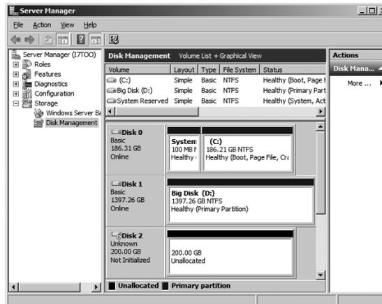
This mounted VHD wasn't formatted as part of the creation process (it hadn't yet been exposed to an operating system installation process). After mounting, you can locate the VHD on the host either by using the Computer Management console or by using the `diskpart` command (see Figure 10.38). Once you identify the volume, you can then perform additional storage tasks from the host.
