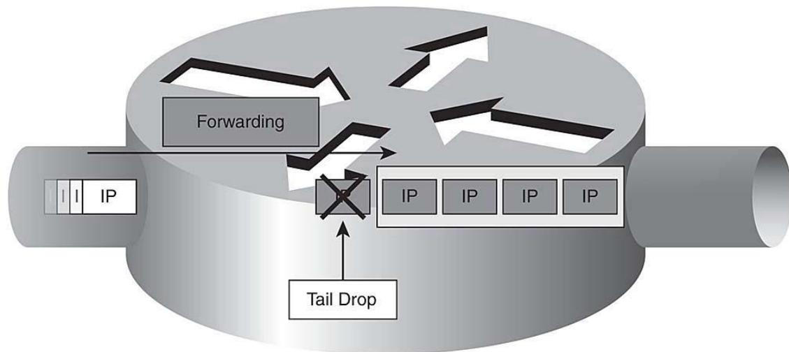
"IP" refers to any type of Internet Protocol (IP) packet in the output queue for an interface.
